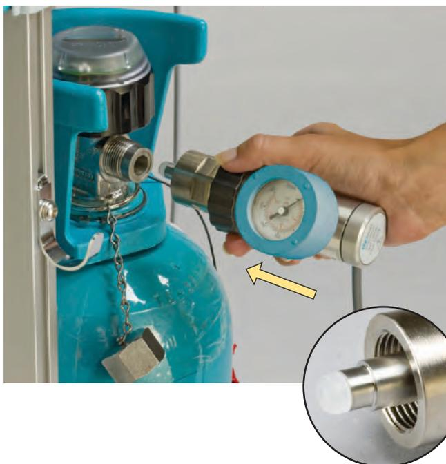
5. Connect an INOMAX regulator to one of the INOMAX cylinders, and hand tighten the fitting to the INOMAX cylinder.
