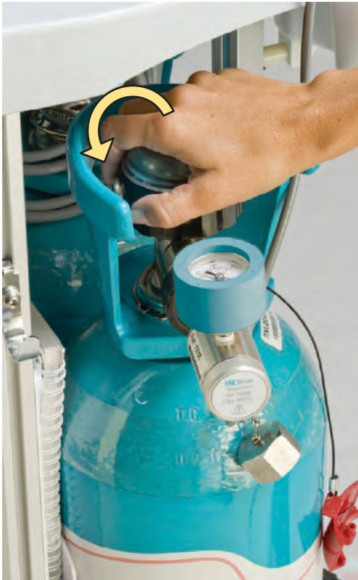
5. Open the cylinder valve on the new cylinder (this may activate the "Two Cylinders Open" alarm until the empty cylinder valve is closed).
