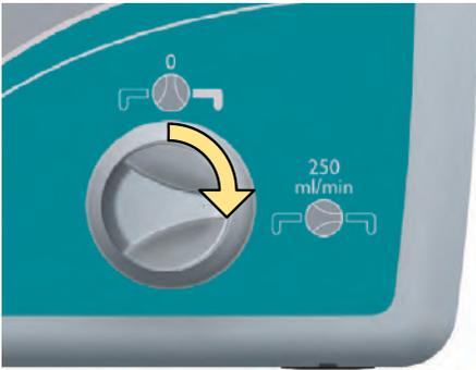
2. Turn the integrated backup INOMAX delivery to ON (250 mL/min.).
