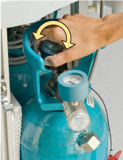
1. Verify one of the high pressure regulators is connected to an INOMAX cylinder.
