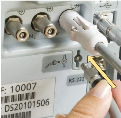
2. At the back of the INOmax DS<sub>IR</sub>, remove the regulator hose from the INOMAX gas inlet and connect it to the purge port.
