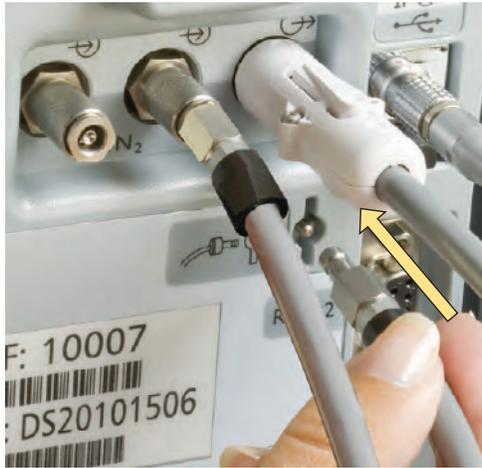
3. Insert the NO/N<sub>2</sub> quick-connect fitting into the purge port on the back of the INOMax DS<sub>IR</sub> and firmly push until the regulator pressure gauge reads zero (this purges any NO<sub>2</sub> that has accumulated in the hose and regulator).
