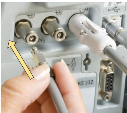
3. When the regulator pressure gauge reads zero, remove the regulator hose from the purge port and connect it to the INOMAX gas inlet.
