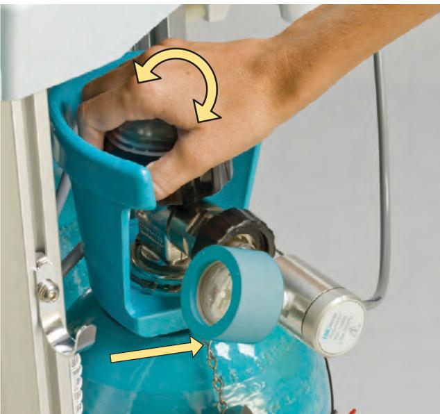
2. Open and then close the valve on the new INOMAX cylinder. Check for adequate cylinder pressure. Monitor pressure gauge for 30 seconds for any signs of leakage. If there is a decrease, check for leaks around the hose connections and cylinder valve connector using soapy water. (see [Section 7/ Maintenance; Cylinder Leak Check](#)).
