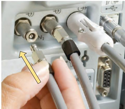
4. Connect the hose to the back (NO/N<sub>2</sub> inlet) of the INOMax DS<sub>IR</sub>. When having difficulty connecting the INOMAX regulator hose, see [page 7-9](#).
